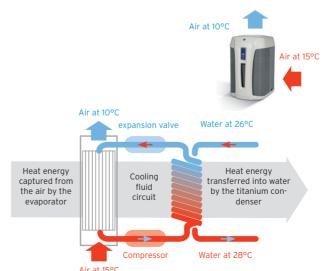
INVERTER technology gives 25 to 45% energy savings (class A) compared to traditional, fixed-speed heat pumps. INVERTER controls and adjusts its speed depending on ambient temperature, in order to obtain the desired temperature.
